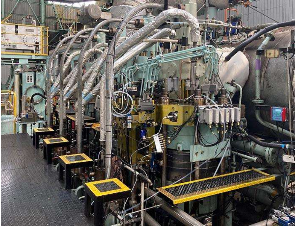
Hydrogen combustion test on MAN B&W 4S50ME-T
