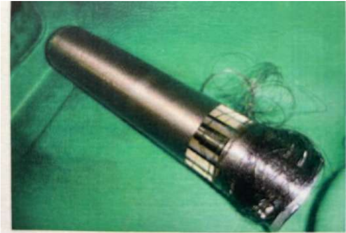
Fig.1 Damaged filter element
