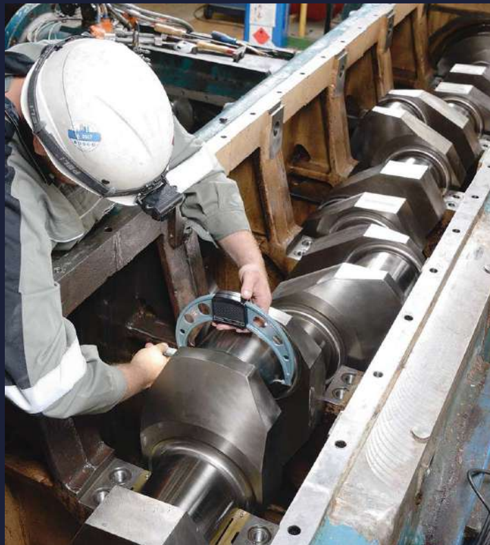
Crankshaft inspection & measurement
