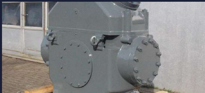
Overhaul of piston compressor
