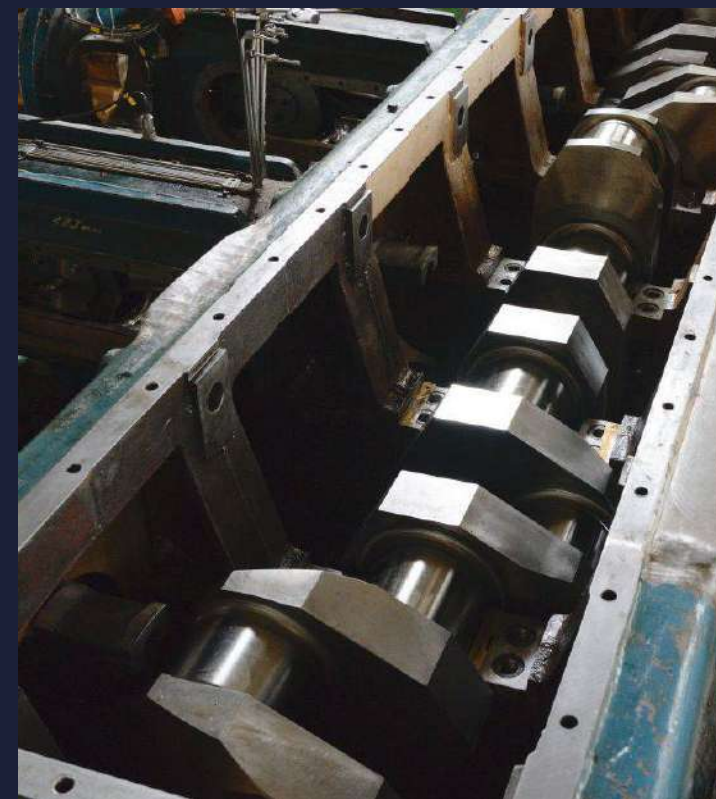
Crankshaft spread measurement
