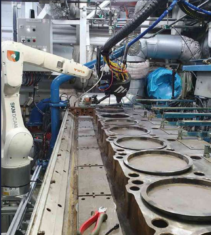
Mobile laser welding
